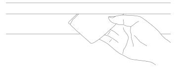
2. For the best wall-washing effect, the light strip should be installed 2-4 inches (5-10 cm) away from the wall surface. Use the provided positioning card for measurement.
